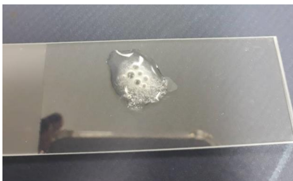
Figure 4. Catalase test showing positive result.
